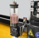
Tech-Sense™ Monitoring System enables true unattended operations. Should the cutting be disrupted the machine will pause the program which can be easily resumed. With our variable feeder, garnet supply is adjusted by the software.
