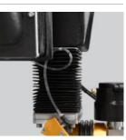
Servo Z axis with auto height position recall, laser terrain mapping (optional) and edge location optics.
