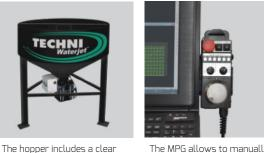
The MPG allows to manually wind forward or backward through a cutting path. This enables the operator to find the exact point along a cutting path from which to re-start cutting after a stoppage, or to simply locate a pre-cut part.
