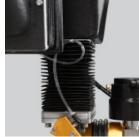
Servo Z axis with auto height position recall, laser terrain mapping (optional) and edge location optics.
