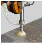
Automatic water Raise/Lower at the push of a button for quieter, cleaner and safer submerged cutting; our tanks include air-tight welds of an air chamber which uses regular shop air pressure.
